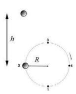
6. [5 marks] A ball of mass 0.5kg attached to a spring (k=800 N/m) is rotating in a horizontal circle from a shaft that makes 5 revolutions every second. The equilibrium length of the spring is 5cm. Calculate the radius of rotation for the ball.
