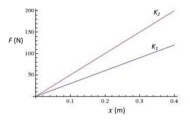
The <u>slope</u> of the line of the F vs. xgraph is the <u>spring constant</u> of the spring.
