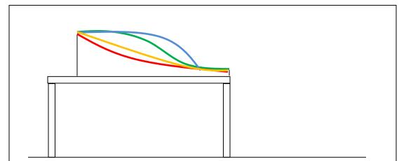
**Qualitative Determination of Launch Speed:** Since all balls leave the table at the same height the horizontal distance at which they land will be a proxy for its horizontal velocity leaving the ramp.
